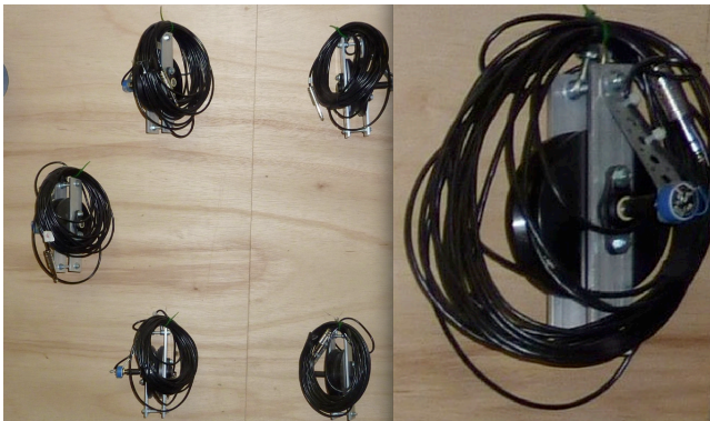
Figure 2. Sensors consisting of wheels, housing, cabling and potentiometers (in blue in the upper right corner detail)
