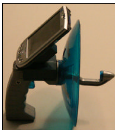
Figure 1.1.1: The gaming device that is used when playing Backseat Playground. The Pocket PC (PDA) is attached to the device itself.
