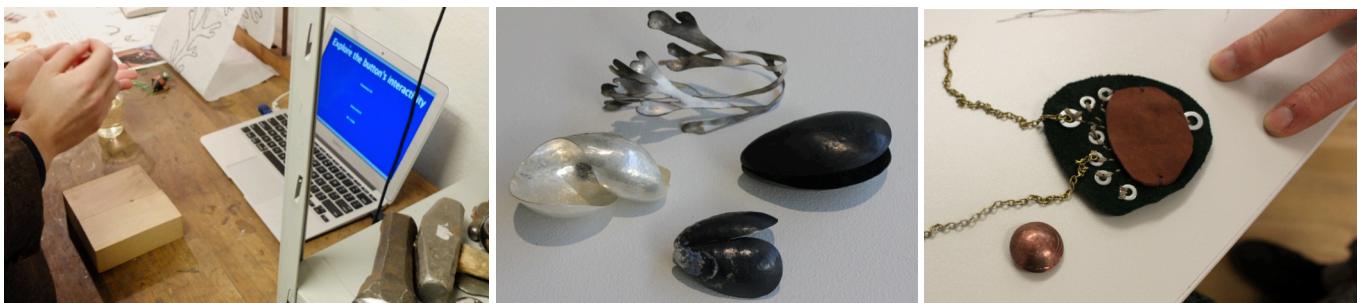
Figure 5. a) A wireless version of a button, demoed in the silversmith studio, in which the touch action was mapped to changing the colour of a laptop screen, b) form study of physical shapes crafted as casings for hosting electronic components of interactive objects, and c) an example of exploring the use of leather for shielding electronics and conductive areas.
