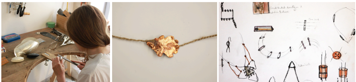
Figure 6. a) The bodily movements performed in silversmith practice informed our focus on designing sensors, b) experiment with single-use button made from copper-coated autumn leaf and copper thread embedded in hemp yarn, and c) example of sketches on how to protect electronics with non-conductive materials and ideas to integrate simple buttons in designs.
